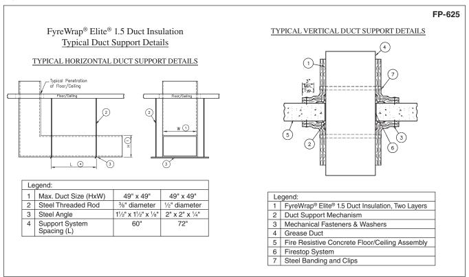
Figure 5. Firestop Installation
